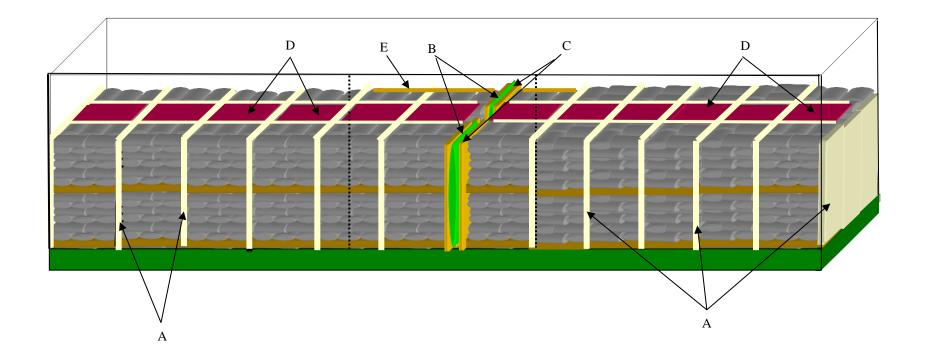
A – PAL-COR FILLER – 4' X 8' X 6" TO REDUCE LENGTHWISE VOIDS B – 48" x 84" X 8 PLY DID BAGS. BAGS TO FIT FACE OF LOAD, KEEP MINIMUM OF 1 INCH OFF OF FLOOR TO PREVENT CHAFFING. C – 4' X 8' X 2" SHEETS OF PAL-COR REDUCING 17" LENGTHWISE VOID TO 8", PROTECTING AIRBAGS D – A 21" LATERAL VOID CONTAINING 2 – 4' x 8' x 2" PAL-COR SHEETS WITH 10" DOR-KOR HONEYCOMB FILLER E – 4' x 8' x 6" PAL-COR BETWEEN LADING AND OFF DOOR
